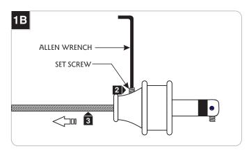
2 Back out (do not remove) the set screw on the connector with the provided Allen wrench.
