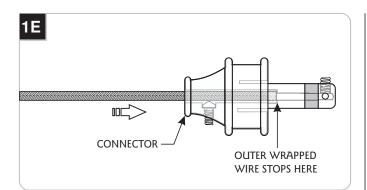
Feed and push the coaxial cable into the connector. The coaxial cable will come to a stop point after being inserted 3/4" into the connector.
