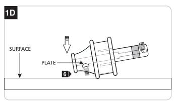
6 Tap the connector on a hard surface with the set screw facing down, so the plate inside drops into place.
