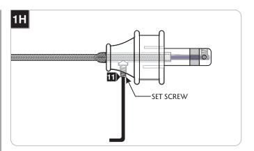
**11** Firmly tighten the set screw on the connector.
