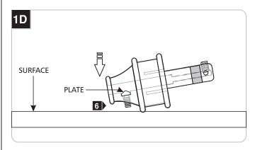
Tap the connector on a hard surface with the set screw facing down, so the plate inside drops into place.
