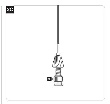
**3** Screw the new lamp into the socket.
