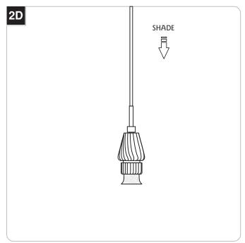
**5** Lower the shade onto the socket assembly.
