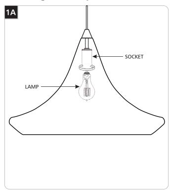
**CAUTION**: To reduce the risk of a burn or electric shock during relamping, disconnect the power to the fixture.
