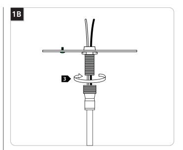
3 Feed the fixture wires through the center of the threaded nipple on the crossbar assembly and screw it completely into the fixture end. Make sure the crossbar is securely tightened.
