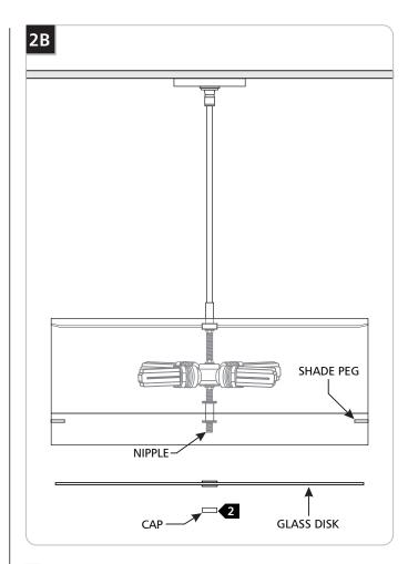
Place the glass disk onto the nipple and secure it against the shade pegs with the cap.
