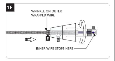
8 Keep pushing the coaxial cable into the connector while rotating the connector to ease feeding the inner wire into the tip of the connector. The outer wrapped wire will start wrinkling while being inserted another 1/2" into the connector.
