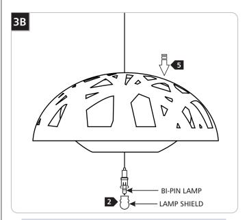
For incandescent versions, use MAX 50 Watt Bi-Pin Halogen Lamp.
