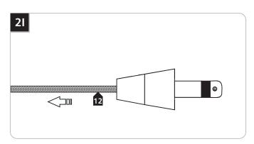
Pull the coaxial cable toward the fixture to smooth the wrinkles.
