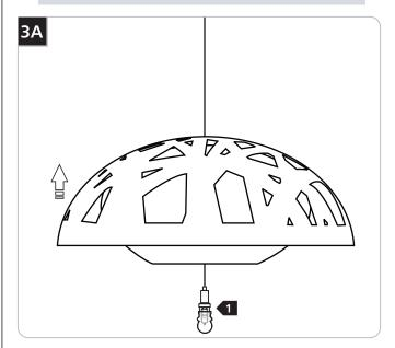
1 Lift the shade assembly up to expose the socket.
