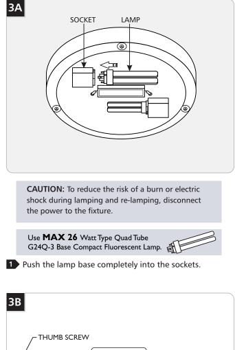
2 Re-install the fixture to the backplate and secure it tightly with the two thumb screws.
