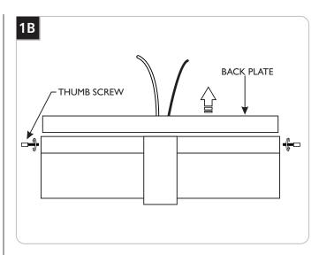
Separate the back plate from the fixture by unscrewing and removing the two thumb screw.
