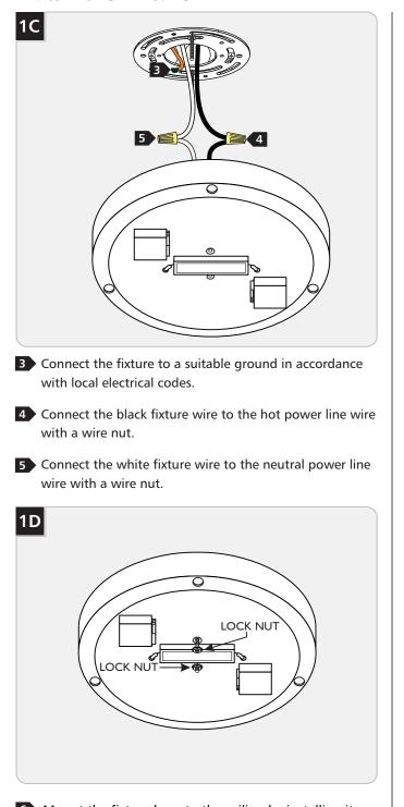
6 Mount the fixture base to the ceiling by installing it onto the mounting plate and securing it tightly with the provided locknuts.
