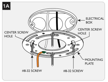
Align the two center screw holes to a wall and secure the mounting plate to the electrical box with the two #8-32 screws provided.
