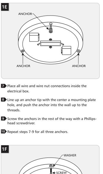
Slide a #8 screw through a washer and screw it into an anchor.
