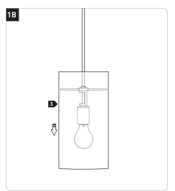
Carefully lower the glass shade to rest onto the socket assembly.
