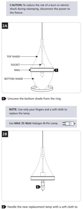
Handle the new replacement lamp with a soft cloth to prevent the natural oils on the fingertips from collecting on the lamp. This will help extend the life of the lamp.
