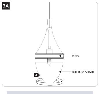
**NOTE:** Do not over tighten the shade. Overtightening may break the glass and result in injury.
