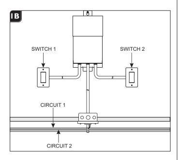
Switch 1 turns on/off Circuit 1 and Switch 2 turns on/off Circuit 2.
