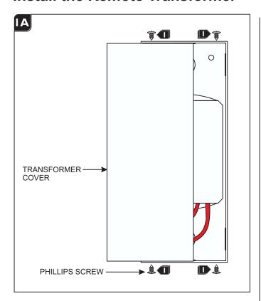
**NOTE:** In order to use small gage wires from the transformer to the electrical box, it is recommended to install the remote transformer near (if possible) the electrical box. See "Low Voltage Wire Size Table" on page 3.
