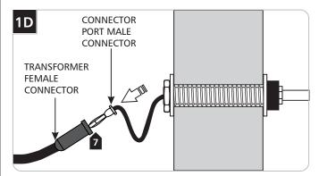
Connect the transformer female connectors to the connector port male connectors.
