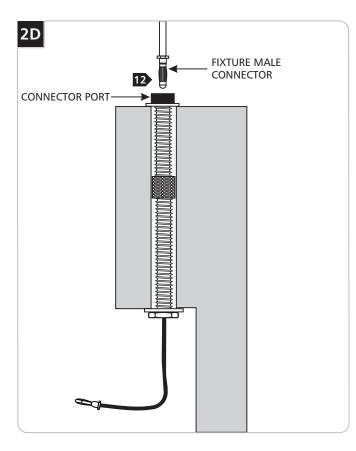
Push the two fixture male connectors completely into the connector ports.
