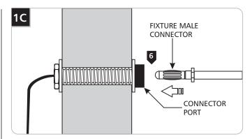
6 Push the two fixture male connectors all the way into the connector ports.
