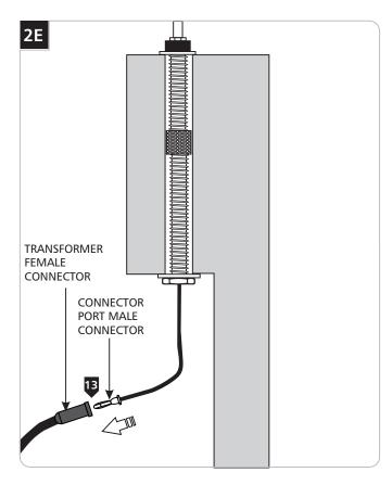
Connect the transformer female connectors to the connector port male connectors.
