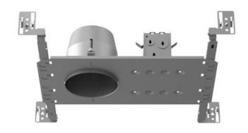
TRIM COLOR N/A **BODY FINISH** Galvanized Steel WATTAGE 50W DIMMER Low Voltage Electronic DIMENSIONS 14.38"L x 7.5"W x 4.5"H **BULB NOT INCLUDED** LAMP MR16/GU5.3 (bipin)/50W/12V Halogen MR16/GU5.3 (bipin)/12V LED Technical Information CEILING TYPE Drywall with Trim HOUSING TYPE New Construction NON IC HOUSING HEIGHT APERTURE SIZE 4.000" SPEC # CLT106642
