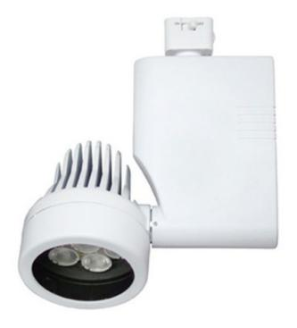
SHADE COLOR N/A BODY FINISH White WATTAGE 27\\\ DIMMER Dimmable DIMENSIONS 3.6"W x 8.5"H x 4.4"D INTEGRATED LED MODULE LAMP 1 x LED/120V LED Technical Information LUMINOUS FLUX 1494 lumens LUMENS/WATT 55.33 COLOR RENDERING 80 CRI 50000 hours LAMP LIFE SPEC # CNT109547
