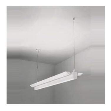
SHADE COLOR N/A BODY FINISH Matte White WATTAGE 240W/ DIMMER Not Dimmable DIMENSIONS 60.234"W x 11.031"H **BULB NOT INCLUDED** LAMP 3 x T5/G5/80W/120V Fluorescent Technical Information LUMINOUS FLUX 6100 lumens LUMENS/WATT 76.25 COLOR RENDERING 95 CRI BEAM ANGLE
