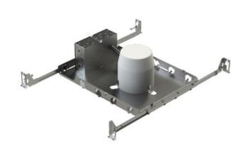
TRIM COLOR N/A BODY FINISH Aluminum WATTAGE 50\\\ DIMMER Dimmable DIMENSIONS 12"L x 6"W x 5.25"H **BULB NOT INCLUDED** LAMP 1 x MR16/GU10/50W/120V Halogen 1 x MR16/GU10/120V LED Technical Information CEILING TYPE Drywall with Trim HOUSING TYPE New Construction NON IC HOUSING HEIGHT SPEC # EUF184744
