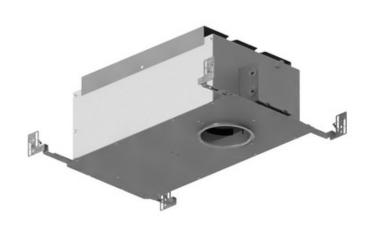
TRIM COLOR N/A BODY FINISH Galvanized Steel WATTAGE 23W DIMMER Low Voltage Electronic DIMENSIONS 19.5"W x 7.1"H x 10"D INTEGRATED LED MODULE LAMP 1 x LED/120V LED Technical Information LUMINOUS FLUX 2000 lumens LUMENS/WATT 86.96 CEILING TYPE Drywall with Trim HOUSING TYPE New construction IC SPEC # CLT234267
