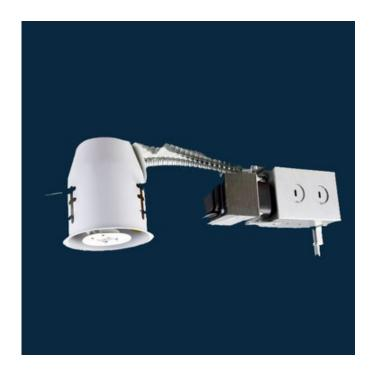
TRIM COLOR N/A BODY FINISH Galvanized Steel WATTAGE 50\\/ DIMMER Dimmable DIMENSIONS 13.5"W x 4.5"H x 3.5"D **BULB NOT INCLUDED** LAMP 1 x MR16/GU10/50W/120V Halogen 1 x MR16/GU5.3 (bipin)/12V LED Technical Information CEILING TYPE Drywall with Trim HOUSING TYPE Remodel NON IC HOUSING HEIGHT 5" SPEC # BEA36925
