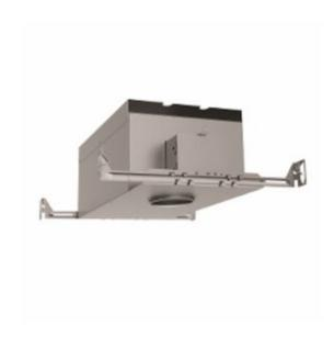
**BODY FINISH** Galvanized Steel 35W/ WATTAGE DIMMER Low Voltage Electronic DIMENSIONS 15.25"L x 8.25"W x 7.9"H **BULB NOT INCLUDED** LAMP 1 x MR16/GU5.3 (bipin)/35W/12V Halogen MR16/GU5.3 (bipin)/12V LED Technical Information CEILING TYPE Drywall with Trim HOUSING TYPE New construction IC Airtight HOUSING HEIGHT APERTURE SIZE 3.500"
