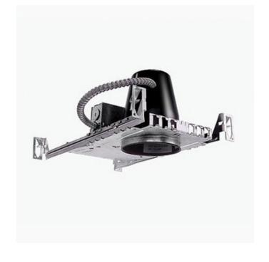
TRIM COLOR N/A BODY FINISH Black WATTAGE 50W DIMMER Low Voltage Magnetic DIMENSIONS 9"L x 11.5"W x 6.31"H **BULB NOT INCLUDED** LAMP 1 x MR16/GU5.3 (bipin)/50W/12V Halogen 1 x MR16/GU5.3 (bipin)/12V LED Technical Information HOUSING TYPE New Construction NON IC HOUSING HEIGHT APERTURE SIZE 4.000" SPEC # WAC55125
