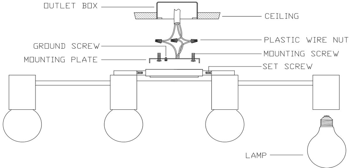
**WIRE NUT/TAPING DIAGRAM**
