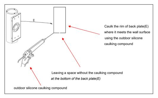
To prevent the water from entering the J-box and causing a short circuit, use the outdoor silicone caulking compound to caulk completely along the rim of back plate(E) where it meets the wall surface, but leaving a space without the caulking compound at the bottom of back plate(E).
