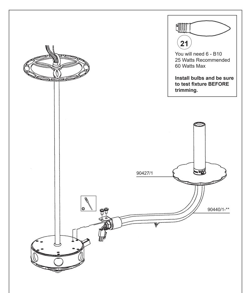
19 Connect arm wires using plug-in connectors. See detailed illustration.
