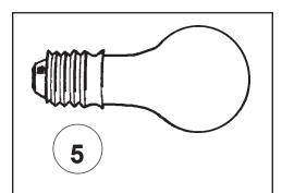
You will need 1 - Type A19 40 Watts Recommended 100 Watts Max MIN 75°C SUPPLY CONDUCTORS
