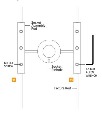
12 Loosen (Do Not Remove) the four M3 set screws on the middle socket assembly rods.
