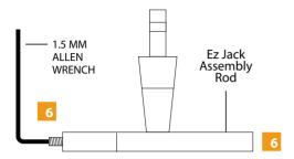
7 Insert the fixture rods into the EZ Jack assembly rod, make sure the fixture rods are aligned with the top of the EZ Jack assembly rod. Tighten the two M3 set screw with 1.5 MM Allen wrench.
