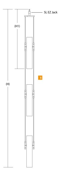
The overall fixture height (H) is measured from bottom of the bottom glass shade to the end of the fixture EZ Jack.
