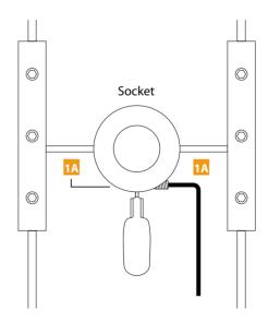
Push the lamp pins completely into the socket holes and tighten the two M3 set screws with the 1.5 MM Allen wrench to secure lamp in place.
