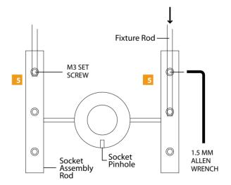
Insert the two fixture rods on the opposite side of socket pin holes, completely into the socket assembly rod and secure into place by tightening the M3 set screws with the provided 1.5 MM Allen wrench.
