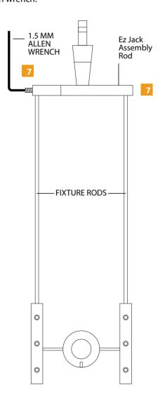
The height (H2) is measured from bottom of the middle glass shade to the middle of the top socket assembly rods. Determine the desired (H2) fixture height. The height (H2) is 39" inches when the fixture rods are not cut.
