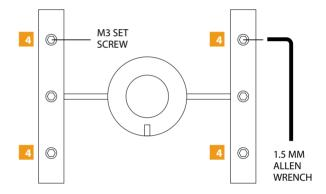
4 Loosen (DO NOT REMOVE) the four M3 set screws on the socket assembly rods.
