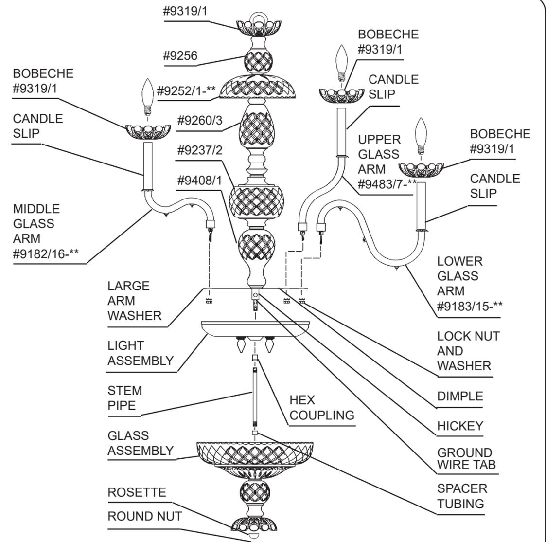
**8** Install upper arms into the inside holes on the washer. **ALTERNATELY** install the middle and lower arms into the outside holes on the washer. **NOTE: THE FIRST LOWER ARM INSTALLED SHOULD LINE UP WITH A UPPER ARM.** Line up holes in arms with dimple in washer. Use lock washer and nut to secure arms in place. Unscrew nut on nipple, place ground wire tab over nipple, secure with nut.
