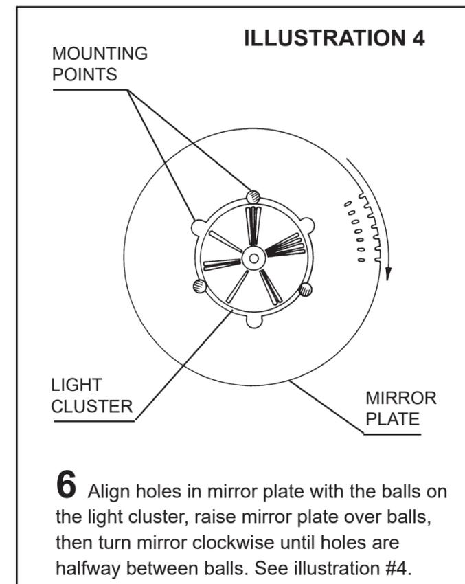
**6** Align holes in mirror plate with the balls on the light cluster, raise mirror plate over balls, then turn mirror clockwise until holes are halfway between balls. See illustration #4.
