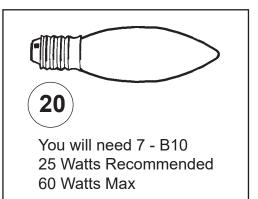
Install bulb and be sure to test fixture BEFORE trimming.
