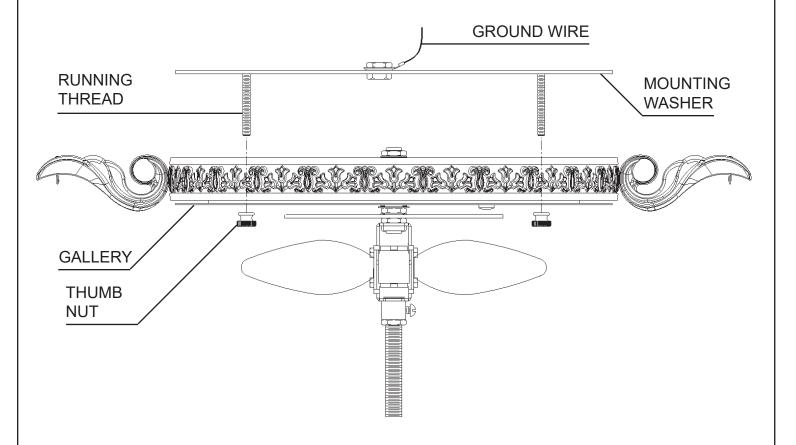
1 Attach mounting washer to outlet box. Connect ground wires from fixture and mounting washer to ground wire in outlet box. Fixture must be grounded. Connect neutral and power wires from fixture to neutral and power wires in outlet box.
