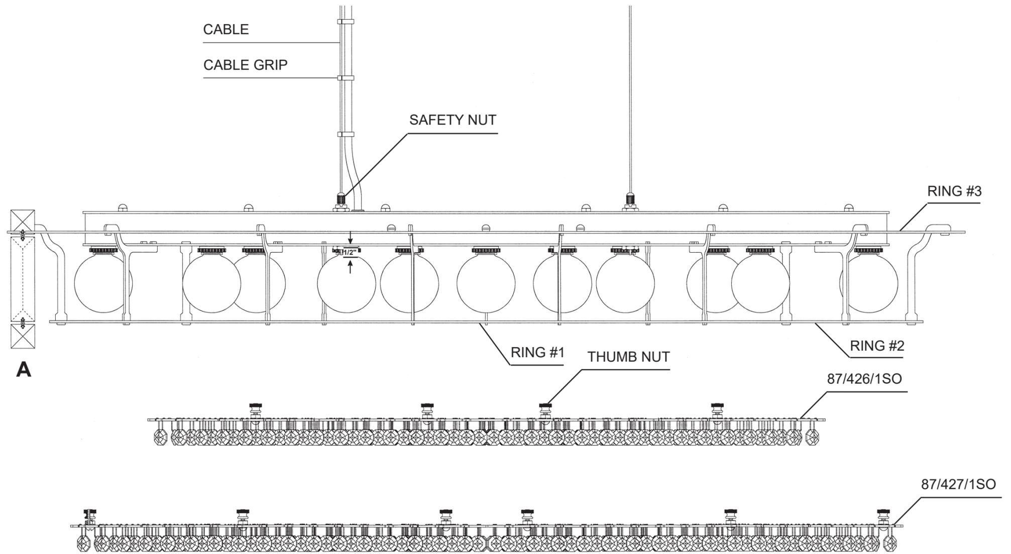
**4** Install two bottom crystal grids with twenty thumb nuts (already screwed onto grids) to bottom of rings #1 & #2.
