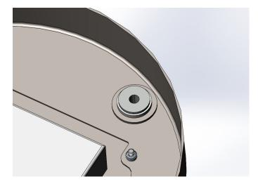
Install **powered** grip-loc cable with **BLACK** end through canopy with swag end inside canopy.
