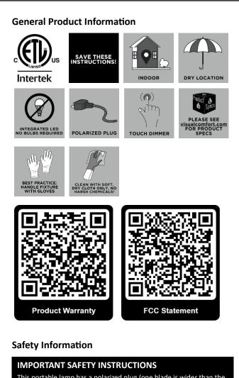
This portable lamp has a polarized plug (one blade is wider than the other) as a safety feature to reduce the risk of electric shock. This plug will fit in a polarized outlet only one way. If the plug does not fit fully in the outlet, reverse the plug. If it still does not fit, contact a qualified electrician. Never use with an extension cord unless plug can be fully inserted. Do not attempt to defeat this safety feature.
