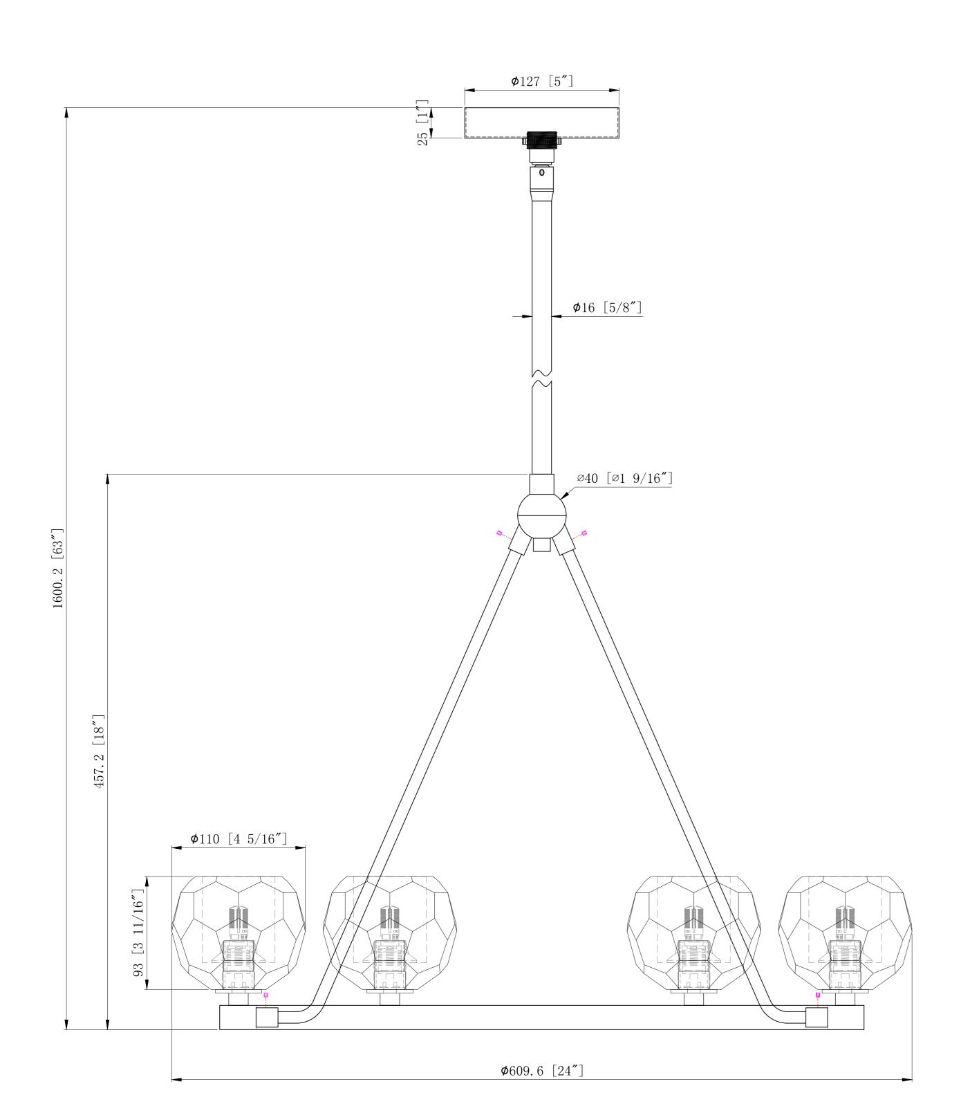
The glass can be installed facing either up or down. Please decide the preferred direction before installing the rod onto the frame.
