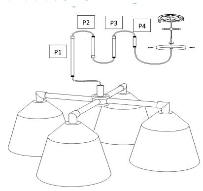
Gently pull the slack cable out of the canopy until the assembled poles meet the thread of the Shade Fixture (H). Screw
