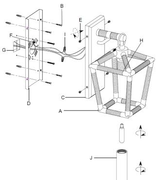
wire is black, and the neutral wire is white. Check to see if there is a ground wire that is either green or green with a yellow stripe or exposed copper metal wire. If needed, use a pair of wire strippers to remove about ½ inch of insulation from each wire
