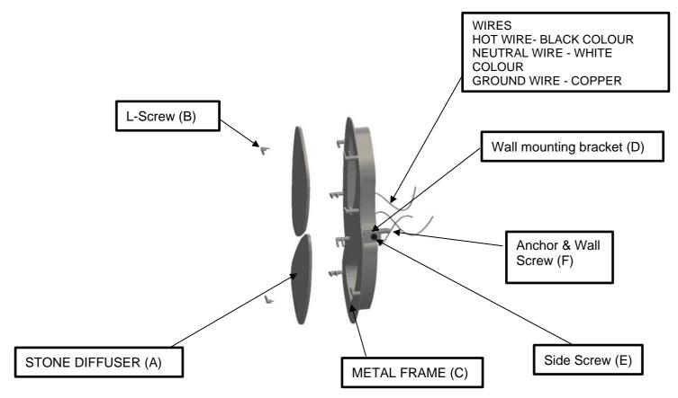
2. Attach Wall Mount Bracket (D) using Anchor & Wall Screw (F).
