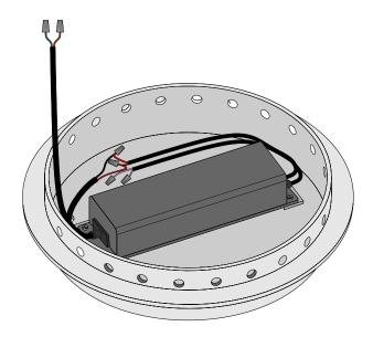
2 - Remove the electrical connections and unscrew the LED driver from the Canopy. Replace new LED driver and attach to the Canopy and establish electrical connections to the appropriate wires. Match specifications of the installed LED Driver. Connect the Fixture wires to the LED driver Output wires (Black) and (Red). Fasten each together with a wire connector and wrap the connection with electrical tape. Be sure that no wire strands are exposed.
