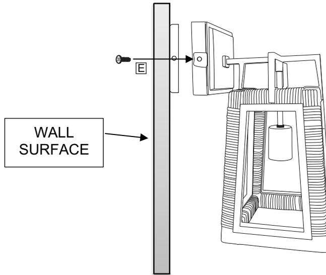
7. Insert One (1) 40 **watt maximum Type A bulb** (not included) into the socket. **DO NOT EXCEED THE RECOMMENDED WATTAGE.** Consider LED Bulbs if brighter light output is desired.
