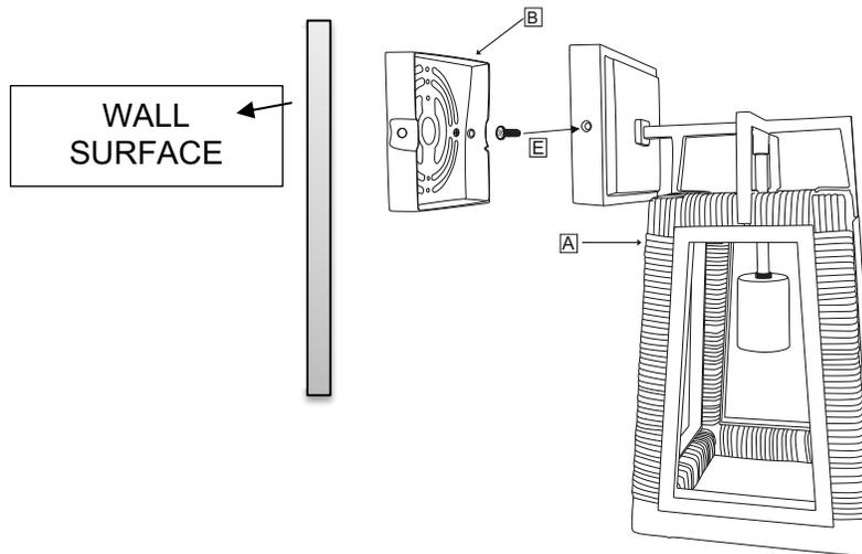
3. Gently pull existing wires out from the wall junction box and allow them to hang. The hot or live wire is often black and smooth or neutral wire is often white and ridged. Check to see if there is a ground wire that is green. If needed, use a pair of wire strippers to remove about 1/2 inch of insulation from each wire.
