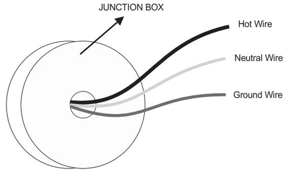
4. Insert the junction box wires through the center opening of the Mounting Plate (B). Attach the mounting plate to the wall Junction Box using the two Mounting Screws (C).
