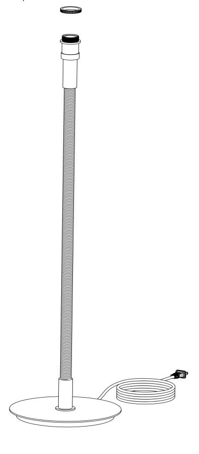
2. Fix the shade then tighten with the washer and insert the E26 bulb in socket.
