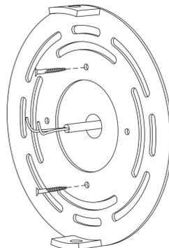
3. Gently pull existing wires out from the wall junction box and allow them to hang. The hot or live & neutral wire is clear. Check to see if there is a ground wire that is copper metal wire. If needed, use a pair of wire strippers to remove about ½ inch of insulation from each wire.
