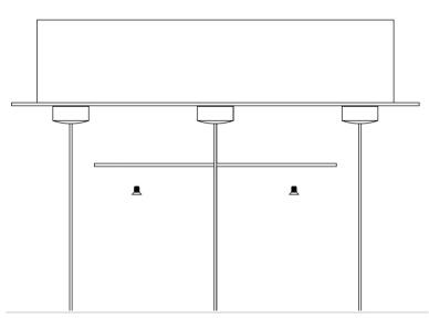
**Step 8**: Install each glass element (G) one by one into female receiver (Gi) ensuring that fixture remains balanced during installation. Glass element is properly installed when snap ring (Gii) locks into place. You may then rotate the glass element freely.
