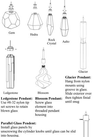
Note that the cylinder knobs do not have to be fully removed from the fixture to install glass panels.
