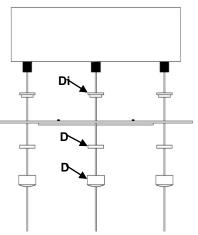
**Step 2:** Mount Canopy (B) to ceiling using the appropriate Hardware Packet (A) and included instructions.
