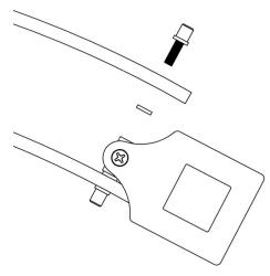
**Note:** The phillips head screws shown in the above image are used to tighten/loosen the glass mounting brackets.
