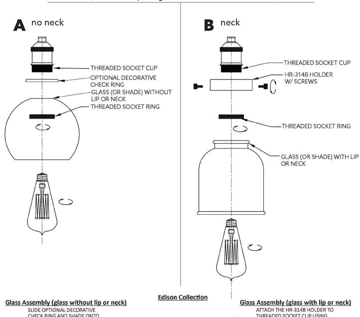
CHECK RING AND SHADE ONTO THREADED SOCKET CUP AND SECURE USING THREADED SOCKET RING
