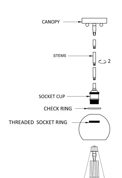
CHOOSE THE NUMBER OF STEMS NEEDED FOR THE CEILING HEIGHT, THEN FEED THE WIRES THROUGH THE STEMS, THEN SCREW THE STEMS INTO THE TOP OF THE FIXTURE AND INTO THE SWIVEL ON THE CANOPY.
