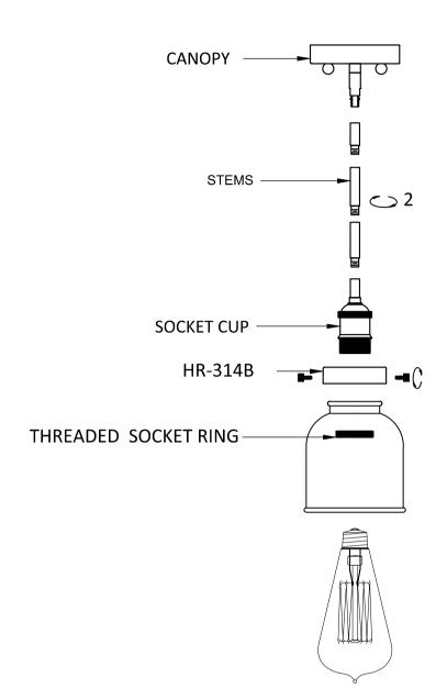
CHOOSE THE NUMBER OF STEMS NEEDED FOR THE CEILING HEIGHT, THEN FEED THE WIRES THROUGH THE STEMS, THEN SCREW THE STEMS INTO THE TOP OF THE FIXTURE AND INTO THE SWIVEL ON THE CANOPY.
