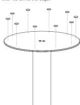
Place the top piece on the column and screw them together with two countersunk screws.
