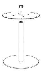
Marble: Align the frame with the threaded holes in the table top. Mount with 6x machine screws. Wood, laminate and glass: Align the frame with the predrilled holes in the table top. Holes may be hidden under felt covering. Mount with 6x wood screws.
