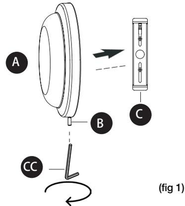
2. Route the junction box wires through the large center hole in the mounting plate (C).
