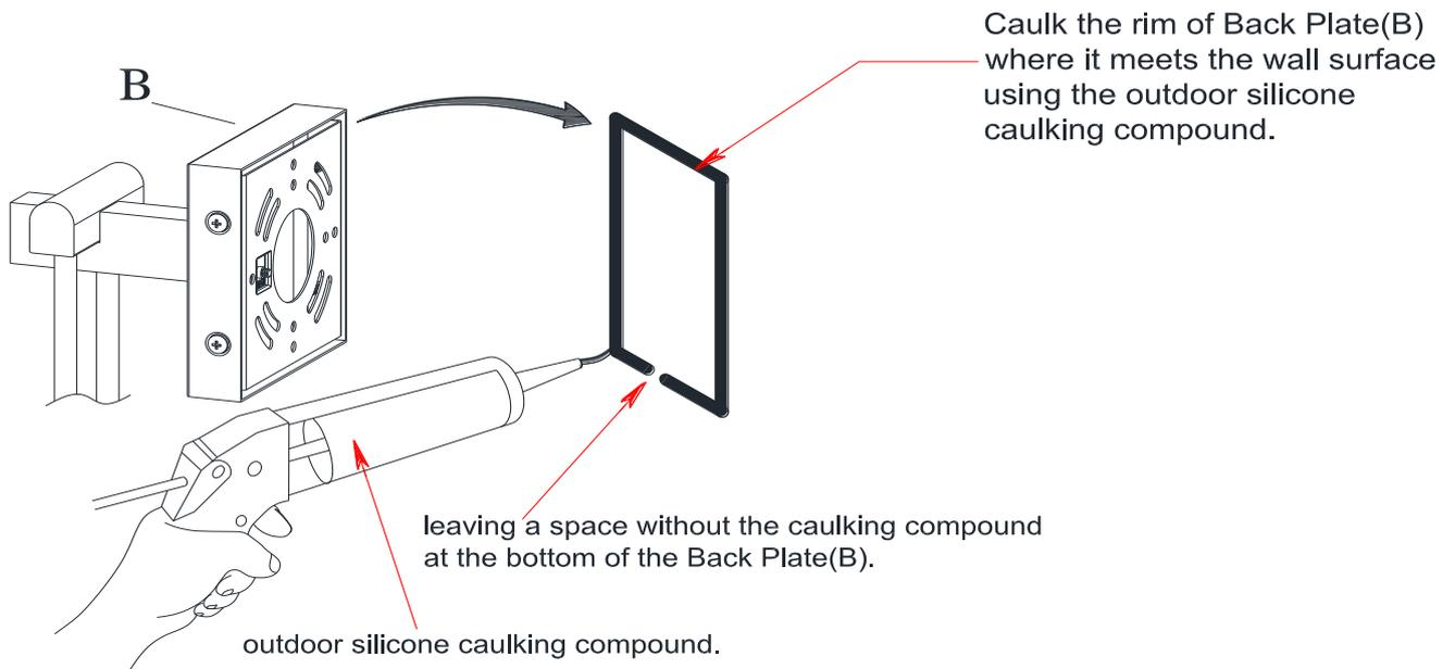
To prevent the water from entering the J-box and causing a short circuit, use the outdoor silicone caulk compound to caulk completely along the rim of Back Plate (B) where it meets the wall surface, but leaving a space without the caulk compound at the bottom of Back Plate (B).
