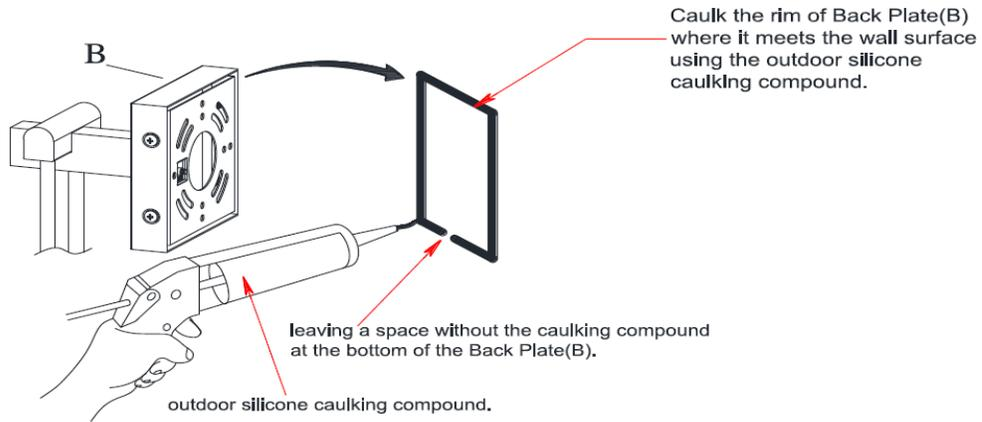
To prevent the water from entering the J-box and causing a short circuit, use the outdoor silicone caulking compound to caulk completely along the rim of Back Plate (B) where it meets the wall surface, but leaving a space without the caulking compound at the bottom of Back Plate (B).
